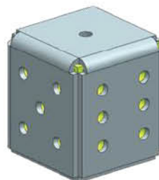
Resulting sheet metal body
