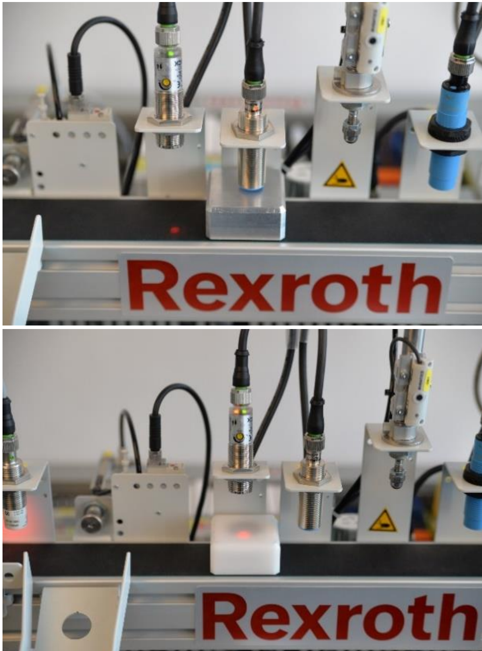
Figure 177: Inductive sensor with aluminum cube (above) and light barrier with plastic cube (below)
