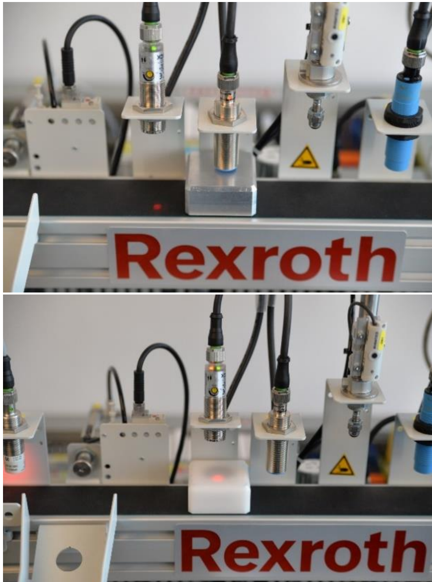
Figure 158: Inductive sensor with aluminum cube (above) and light barrier with plastic cube (below)
