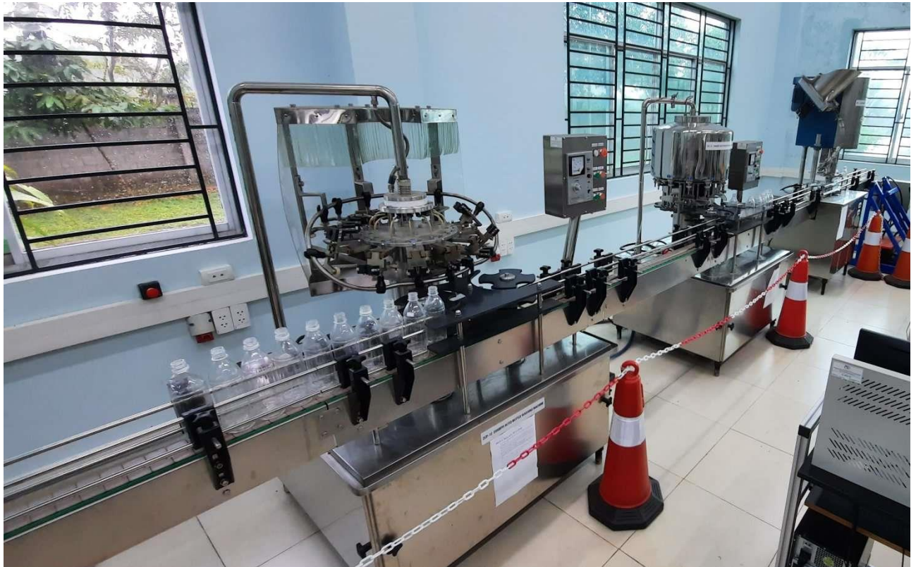
Figure 179: Bottling station full setup, cleaning(left), filling (middle) and capping (right)
