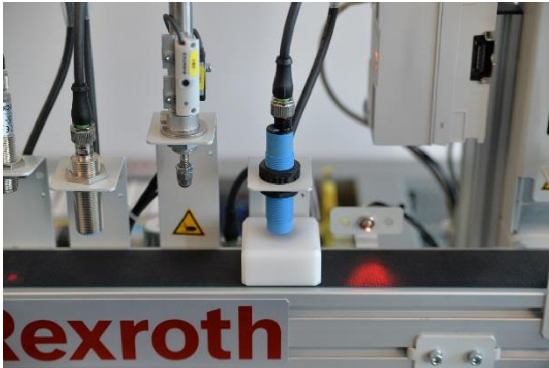
Figure 175: Cube detected by capacitive sensor
