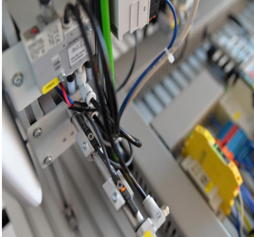
Figure 173: Magazine cylinder with two reed contacts
