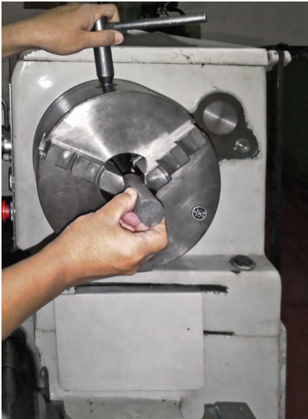
Figure 14. Setting an object on a chuck
